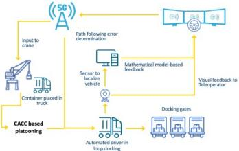
Fig. 3. UC2 sequence including automated docking and teleoperation of a crane.
