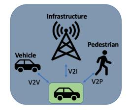
Fig. 1. Some examples of different types Vehicular communications.
