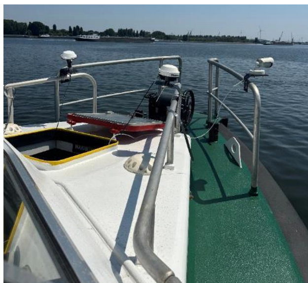
Figure 21 Two GNSS receivers and one camera installed on the boat.
