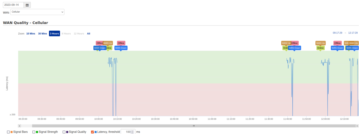
Figure 39 Latency when connected to 5G SA sim on test T1.5
