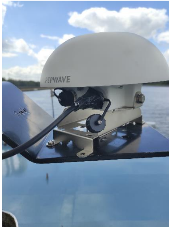
Figure 3 The new modem used for 5G NSA and SA connectivity.
