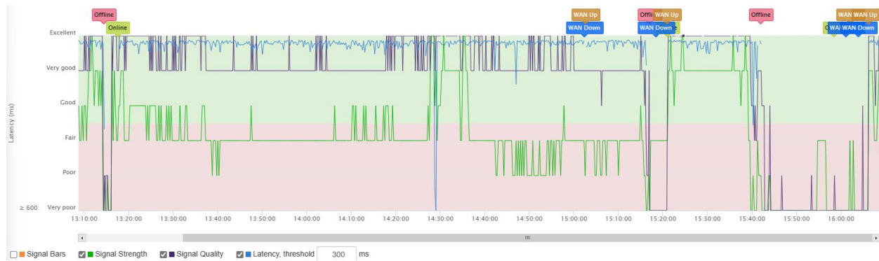
Figure 64 5G SA signal quality while connected with KPN sim card and crossing the border with car.
