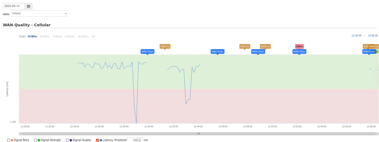
Figure 40 Latency when connected to 4G/5G NSA sim on test T1.5
