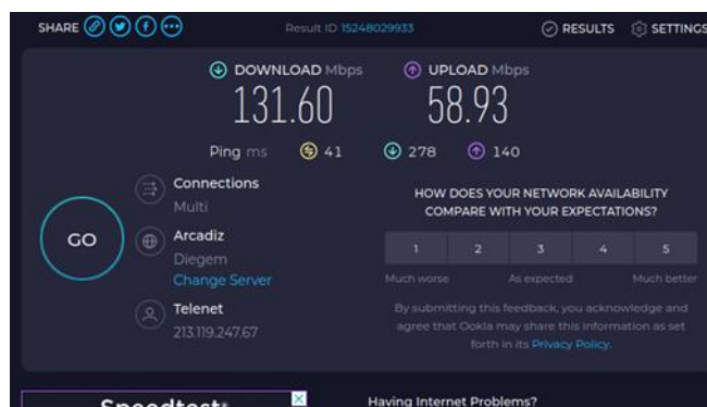
Figure 32 BW test after switching to 4G/5G NSA sim
