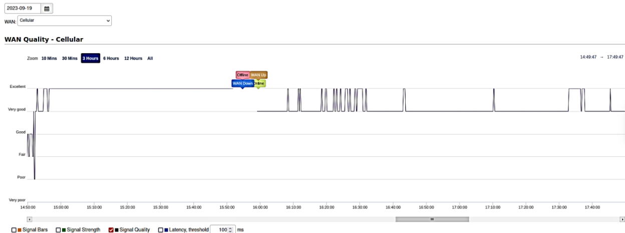
Figure 43 5G SA signal quality during sailing in T2.6
