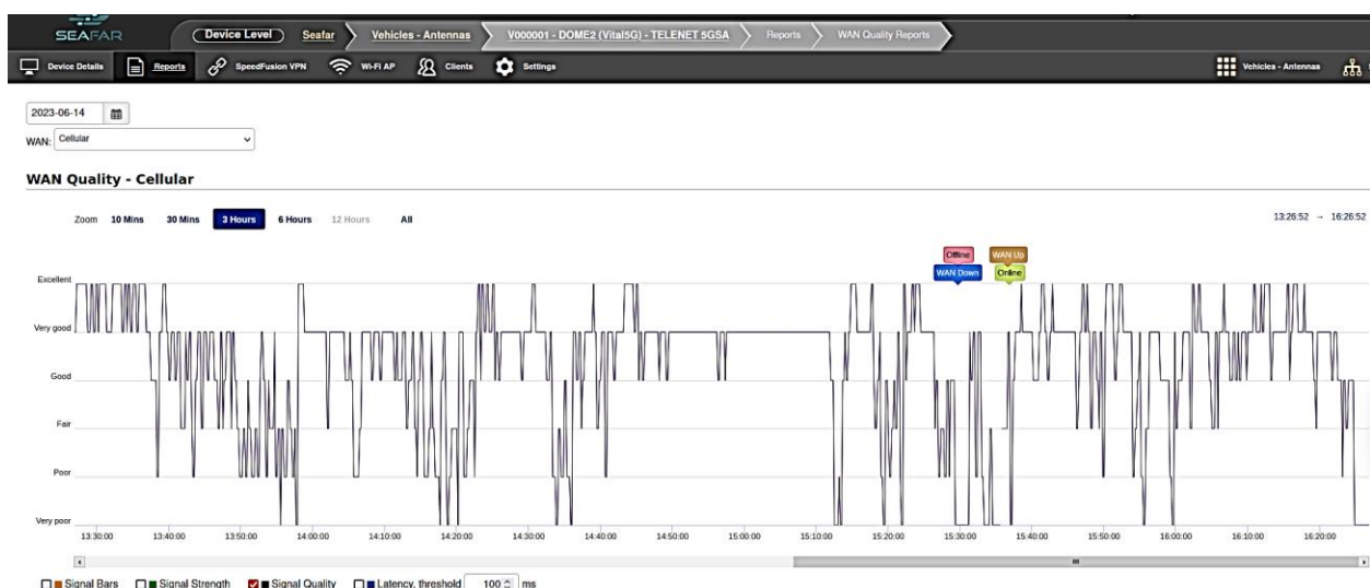
Figure 27 5G SA WAN quality based on signal quality on boat at Port of Antwerp
