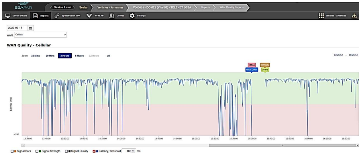
Figure 28 5G SA latency on boat at Port of Antwerp
