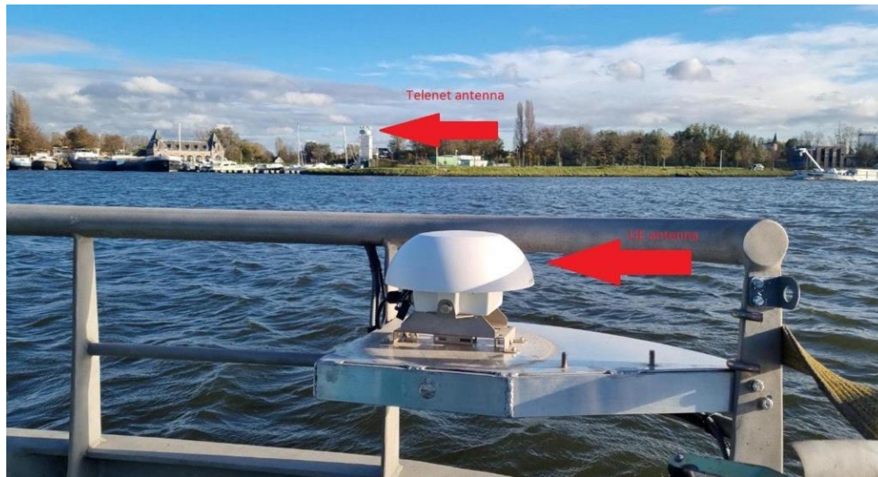
Figure 70 Railing of the urban barge preventing the LoS communication with the base station.
