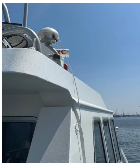
Figure 22 5G modem installed on top of the boat.
