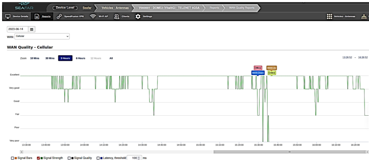
Figure 26 5G SA WAN quality based on signal strength on boat at Port of Antwerp
