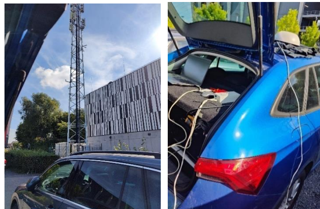
Figure 30 Car equipped with 5G modem parked under Telenet base station to test the connectivity.
