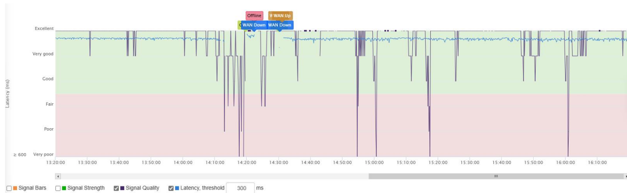
Figure 68 5G SA signal quality connected with Telenet simcard and sailing across the border.
