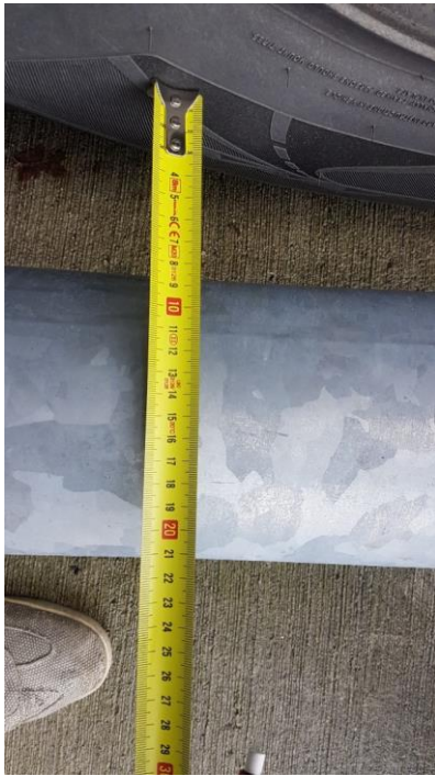
Figure 39: Clearance left side ( \pm 8.5 cm).
