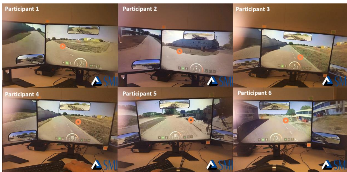
Figure 56: Compilation of stills from eye-tracking device illustrating the drivers' attention to the sides of the road in order to decide the position of the truck.
