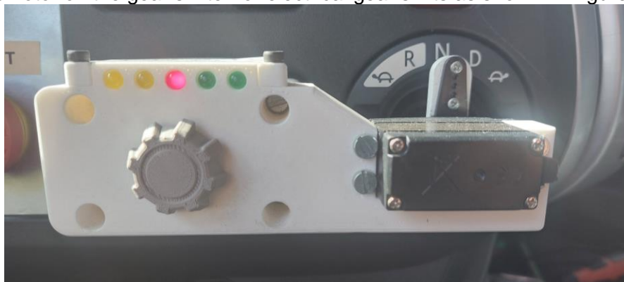
Figure 13: Servomotor with 3D printed mount on original gear shifter.
