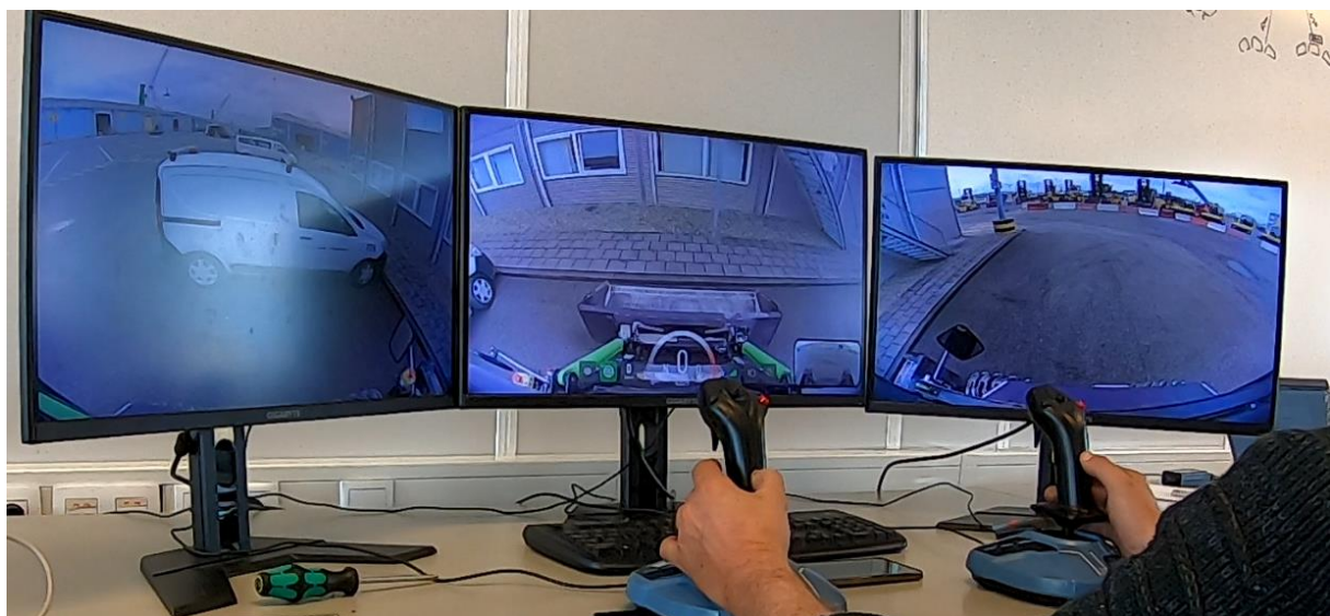
Figure 60: Simplified teleoperation set-up for Skid-Steer driving, including the joysticks & camera streams.
