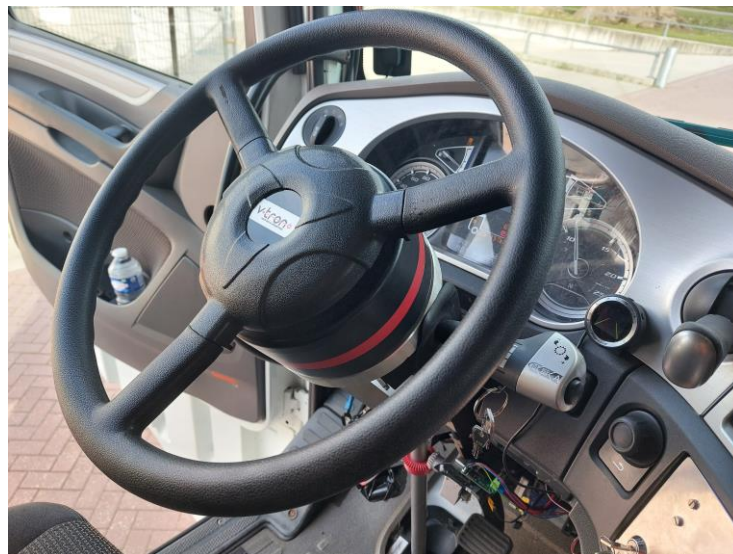
Figure 11: Electrical motor under steering wheel for electric steering control.
