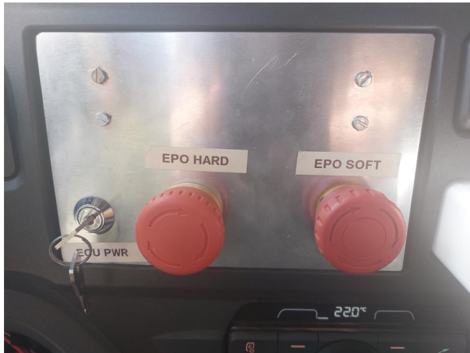
Figure 14: Emergency buttons ('hard' and 'soft' shut-off).
