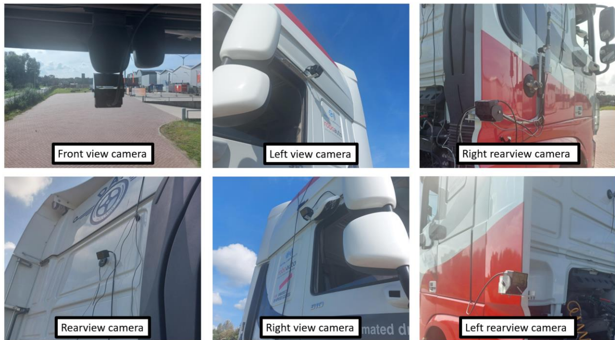
Figure 16: Camera mounting positions.
