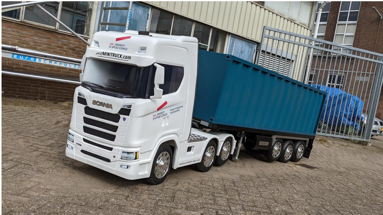
Figure 7: 1:3 Scaled truck and trailer combination used for first developments and MVP testing.
