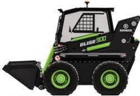
Figure 59: Skid steer loader Elise 900 from Firstgreen Industries, used for teleoperation.
