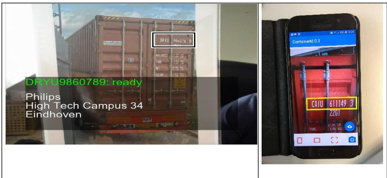
Figure 15: Container ID recognition with overlay
