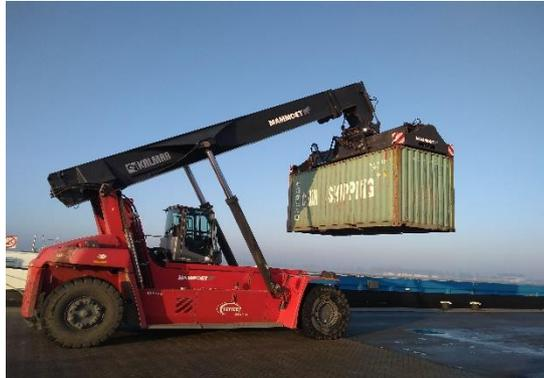
Figure 16: Picture of a reach stacker
