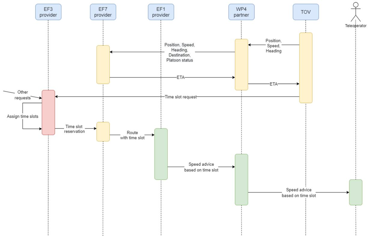
Figure 8: Sequence diagram EF3 iTLC - secondary channel
