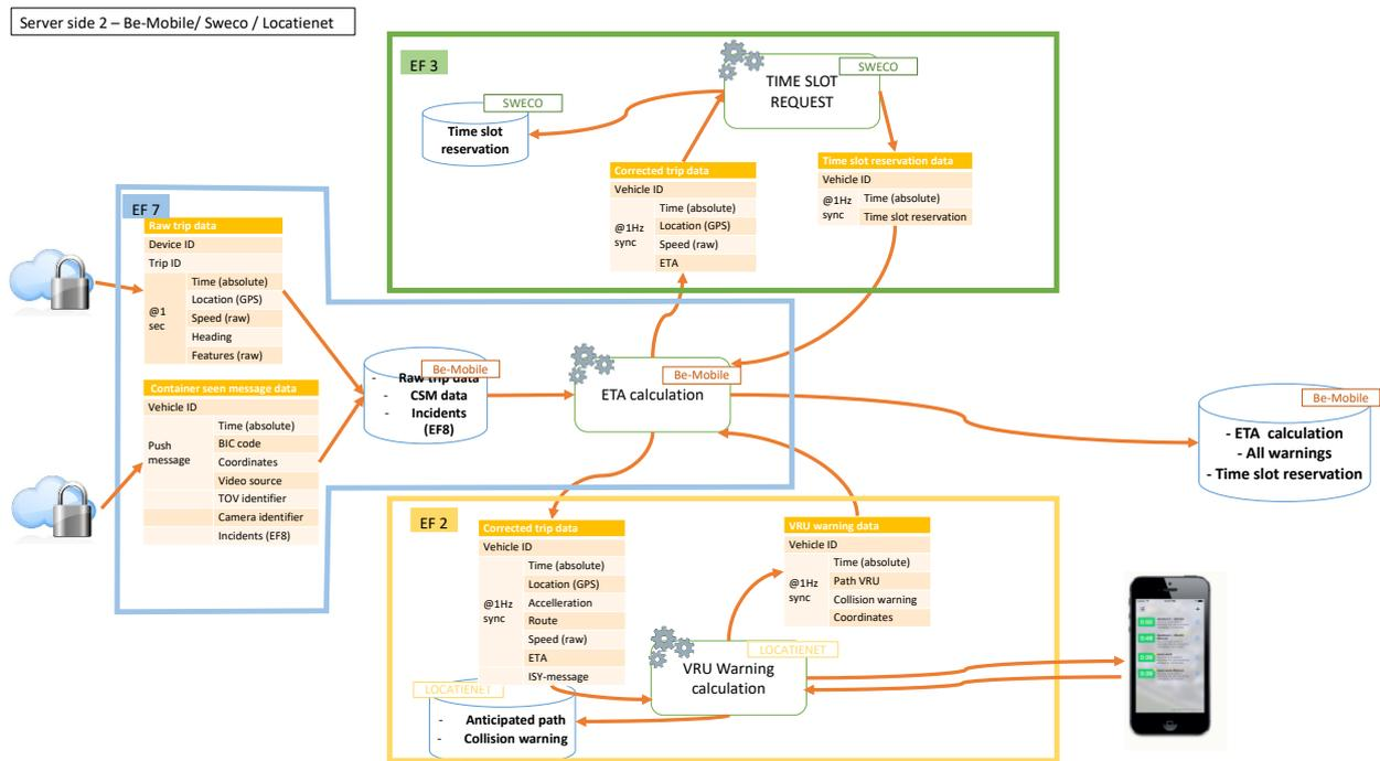
Figure 24: Data processing by EF2 VRU, EF3 iTLC and EF7 ETA
