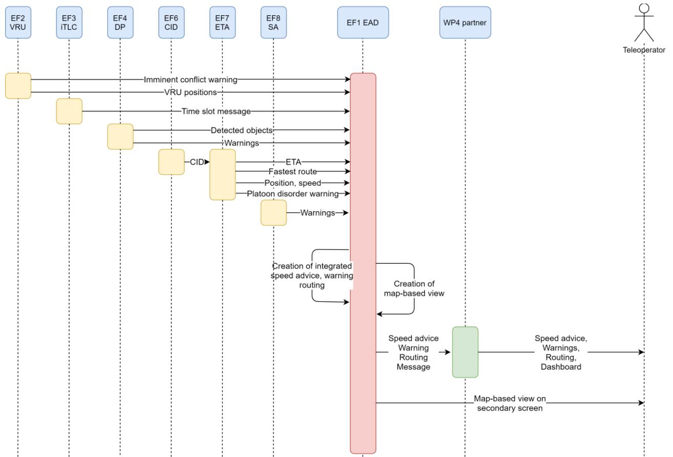
Figure 2: EF1 EAD Sequence Diagram
