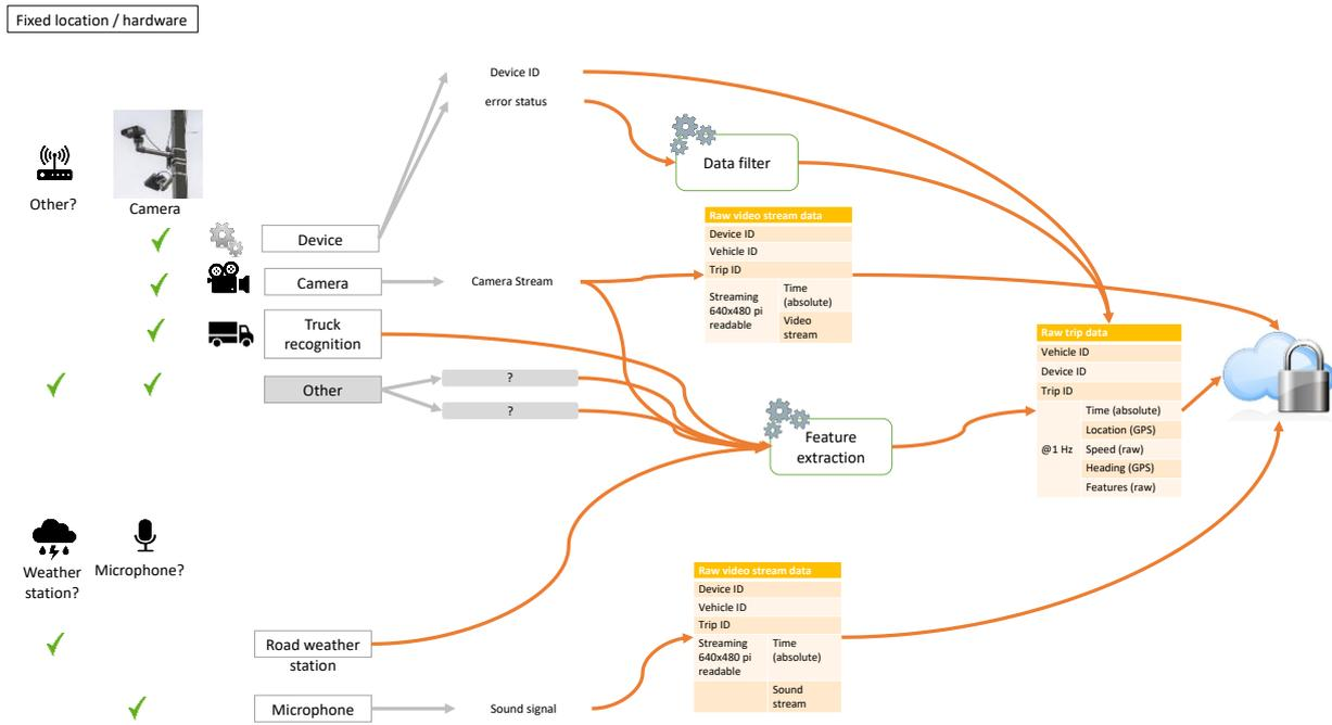
Figure 22: Sensors and data collected from other hardware and fixed locations
