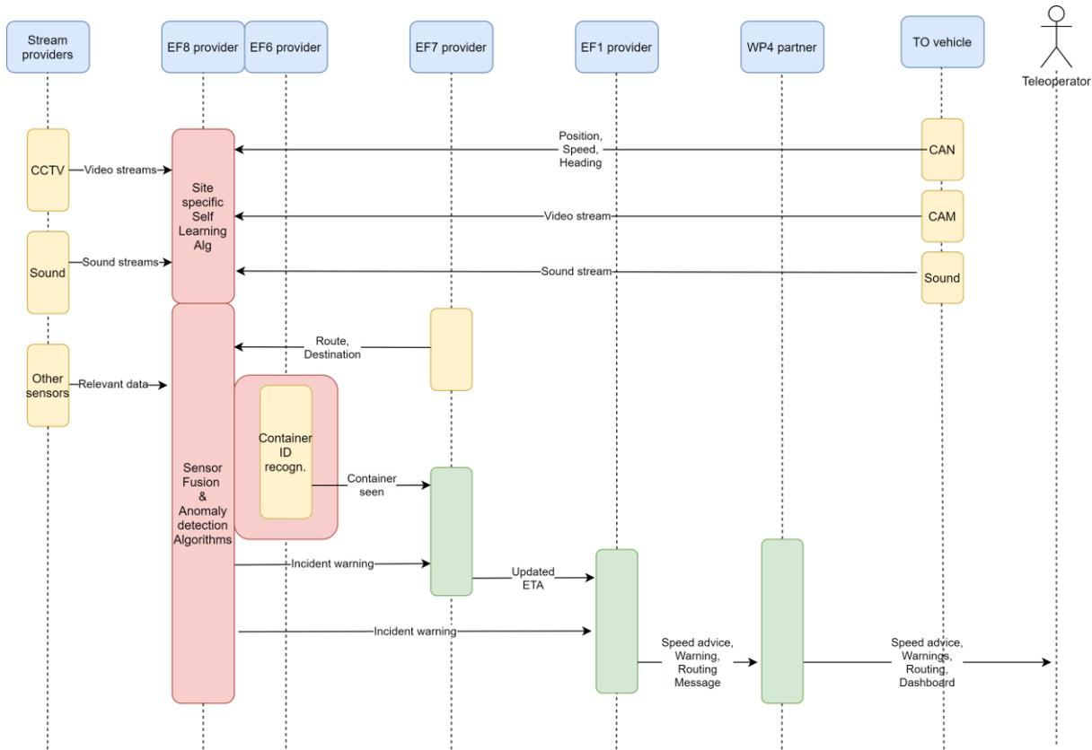
Figure 19: Sequence diagram for EF8 SA
