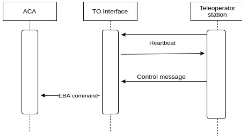
Figure 11: Connection between ACA and teleoperator station
