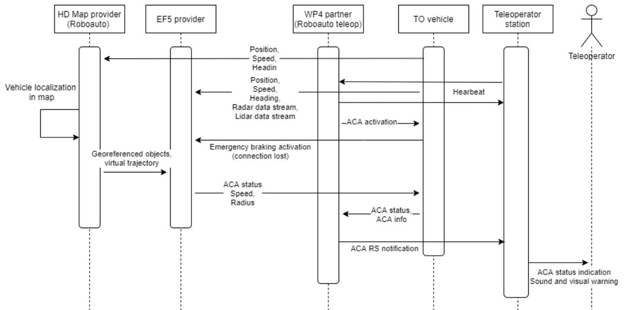
Figure 13: Sequence diagram for EF5 ACA
