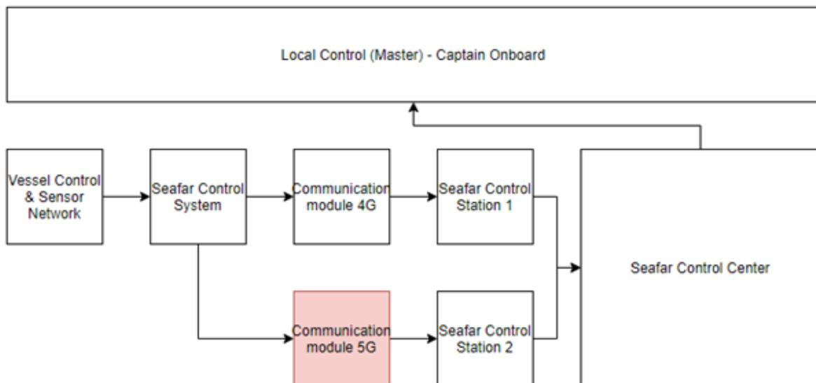
Figure 3: Automated barge control process flow
