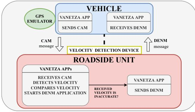
Fig. 5: Entities, Vanetza applications, velocity detection, and messages
