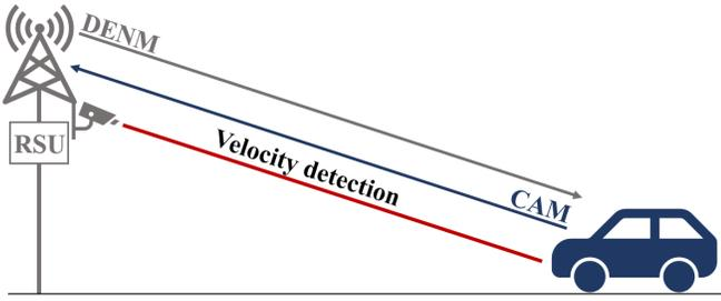
Fig. 1: Velocity detection and C-ITS messages
