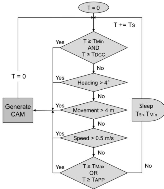
Fig. 3: CAM generation from a vehicle [15]
