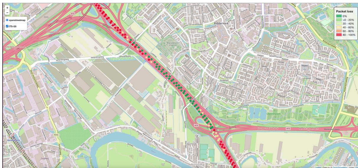
**Figure 11 – Packet Loss on an RSU during the Test Campaign in Netherlands Test Site**
