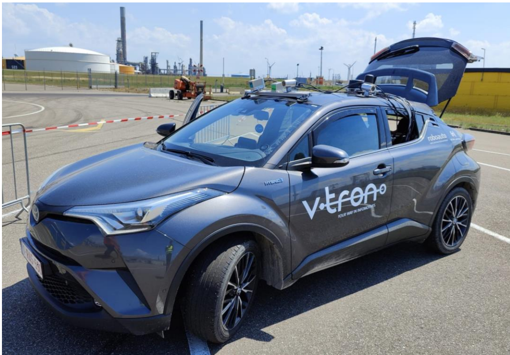
Figure 11 - Pilot vehicle with teleoperation cameras installed
