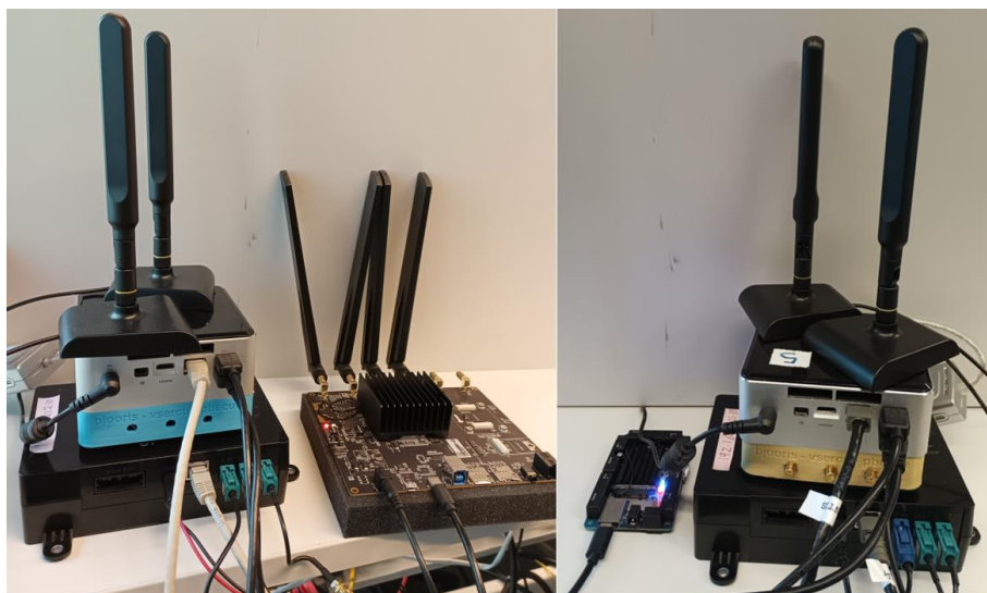
Figure 21: The two nodes of IDLab's V2X test setup.
