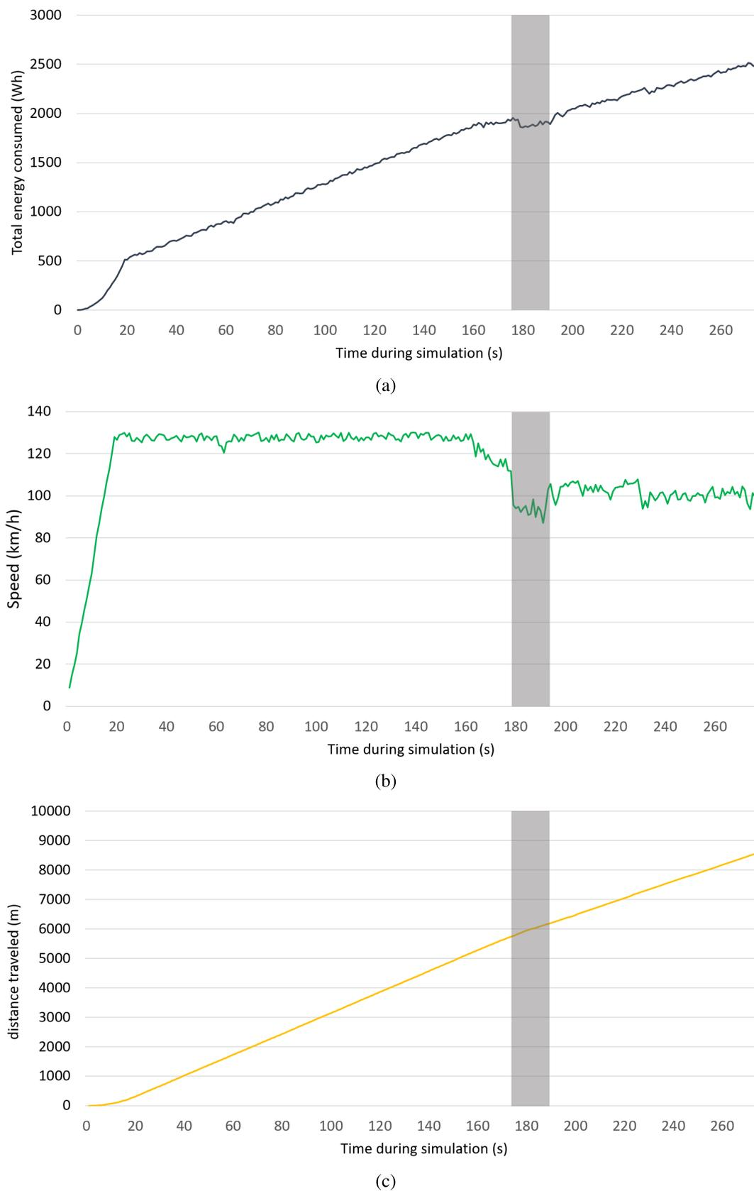
**FIGURE 4.** Example of a single EV traveling on a highway layout: (a) energy consumed during the simulation, (b) speed of the selected vehicle, and (c) distance traveled.
