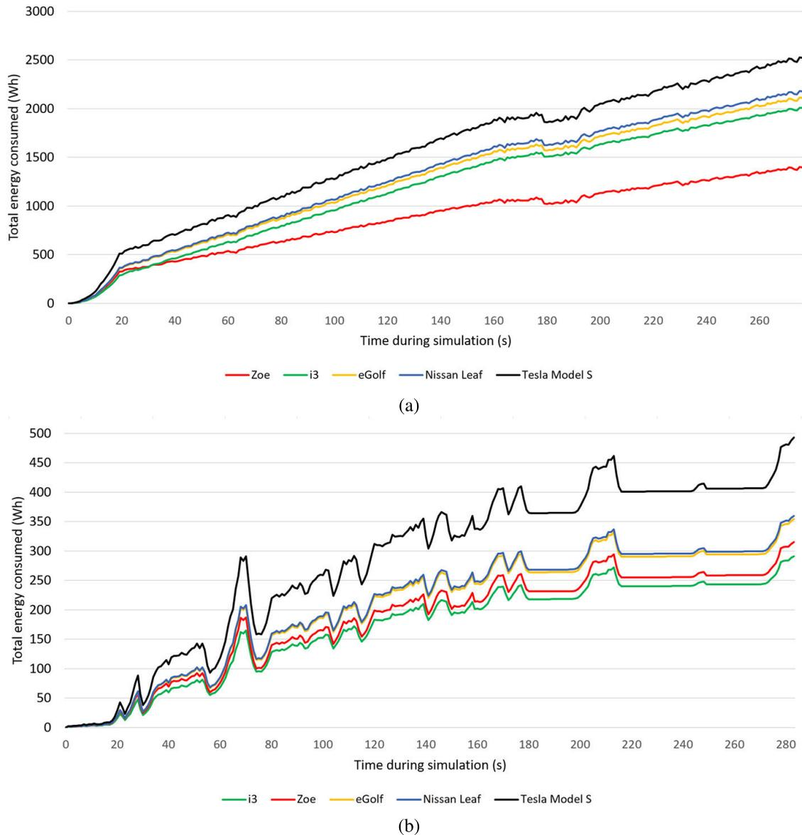
**FIGURE 6.** Comparison of different EV models consumption at: (a) Highway layout and (b) Urban layout.
