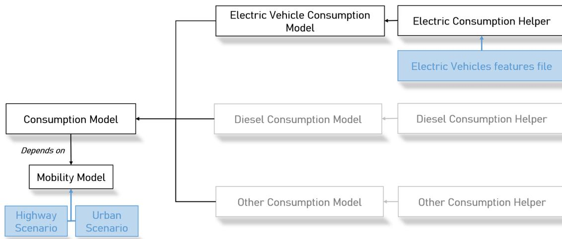
FIGURE 3. Software structure following the ns-3 code guidelines including files needed for the simulation (in blue).
