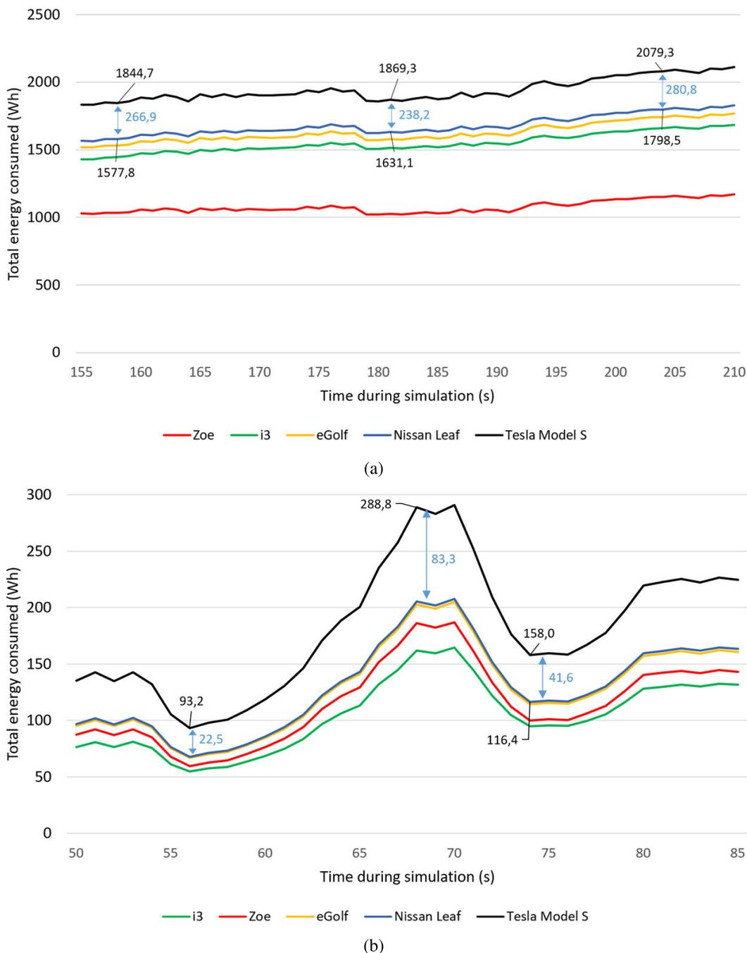
FIGURE 7. Details of different EV models consumption at: (a) Highway layout and (b) Urban layout.
