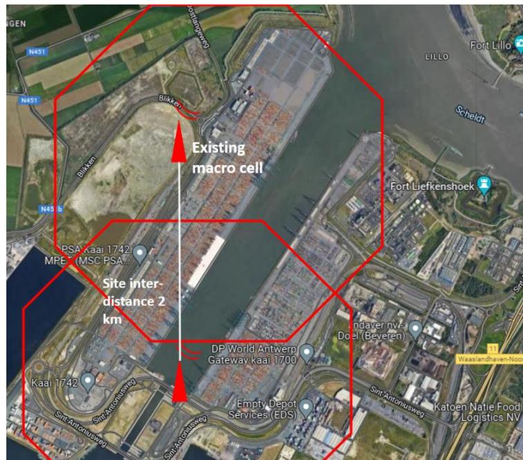
Figure 16 5G network deployment to cover DPW terminal
