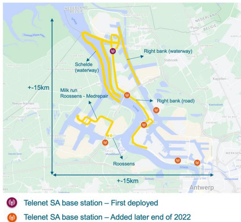
Figure 5 Iterative deployment of 5G NR in the Antwerp pilot site.
