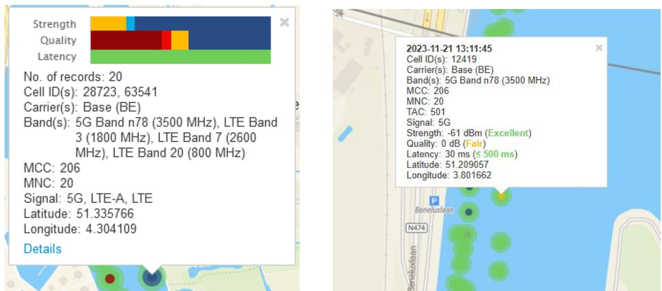
Figure 21 Example of color code for the measurements a) during a test in Port of Antwerp, and b) during a test in Zelzate.
