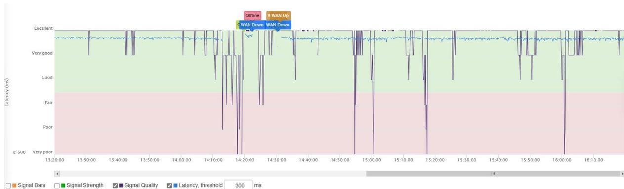
Figure 32 5G SA signal quality connected with Telenet SIM card and sailing across the border in T2.6.
