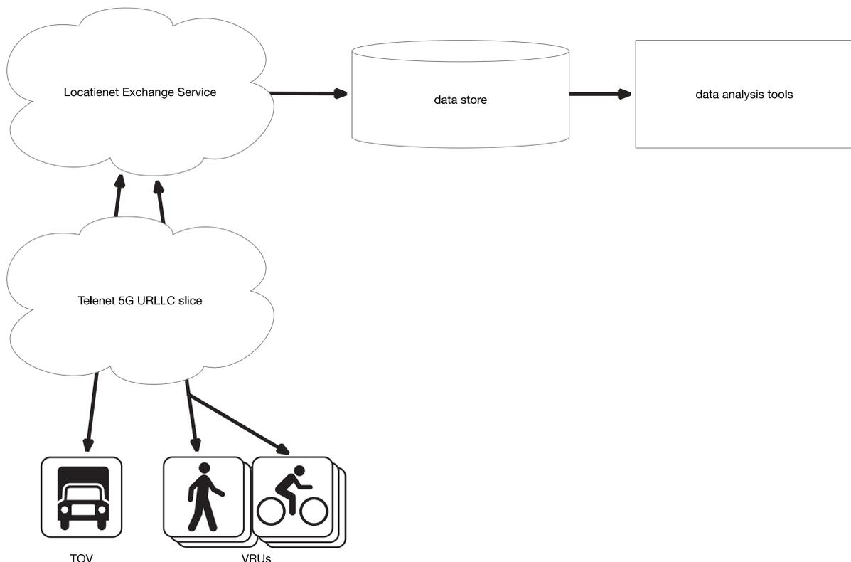
Figure 41 Setup for the logging of messages and network characteristics for analysis.
