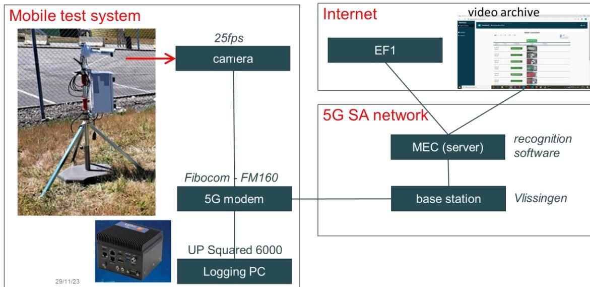
Figure 64 EF6 system setup.
