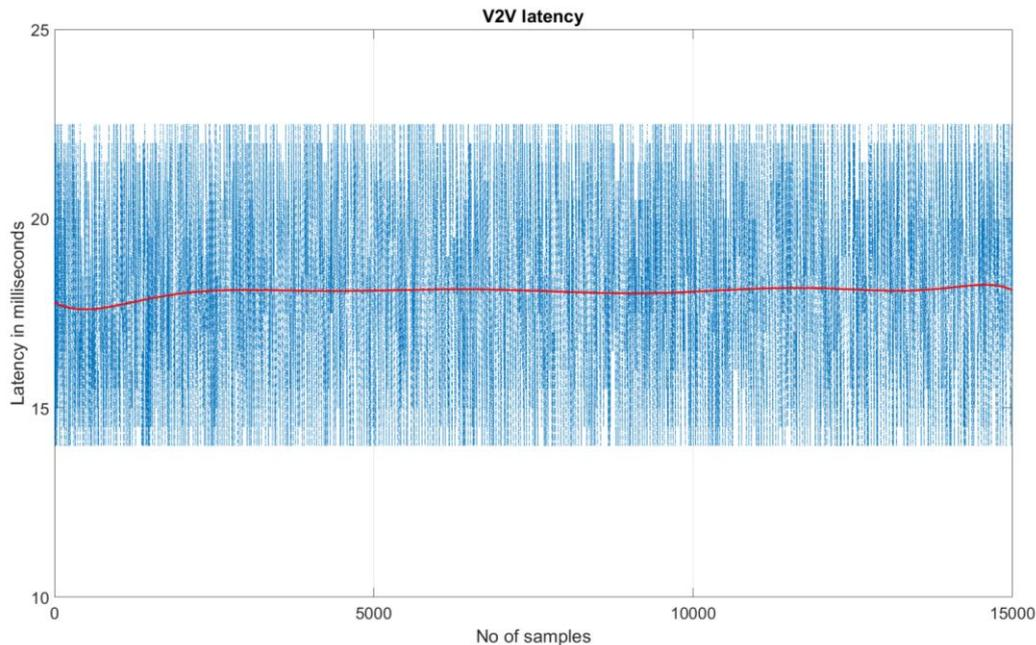
Figure 10 V2V latency plot for CACC-based platooning in Vlissingen.
