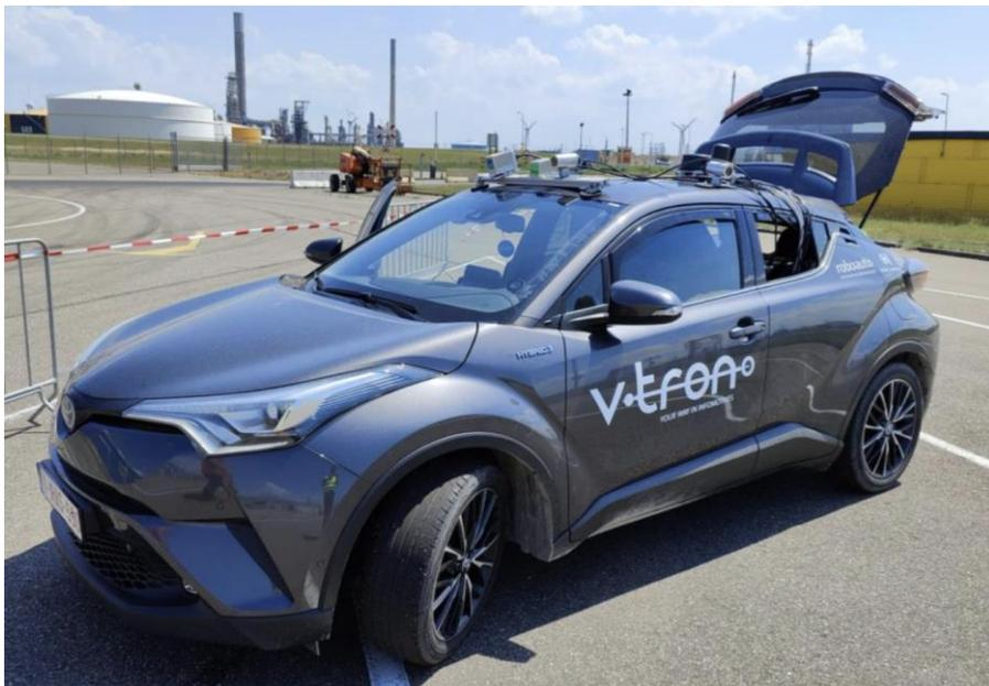
Figure 8 Pilot vehicle with installed cameras.
