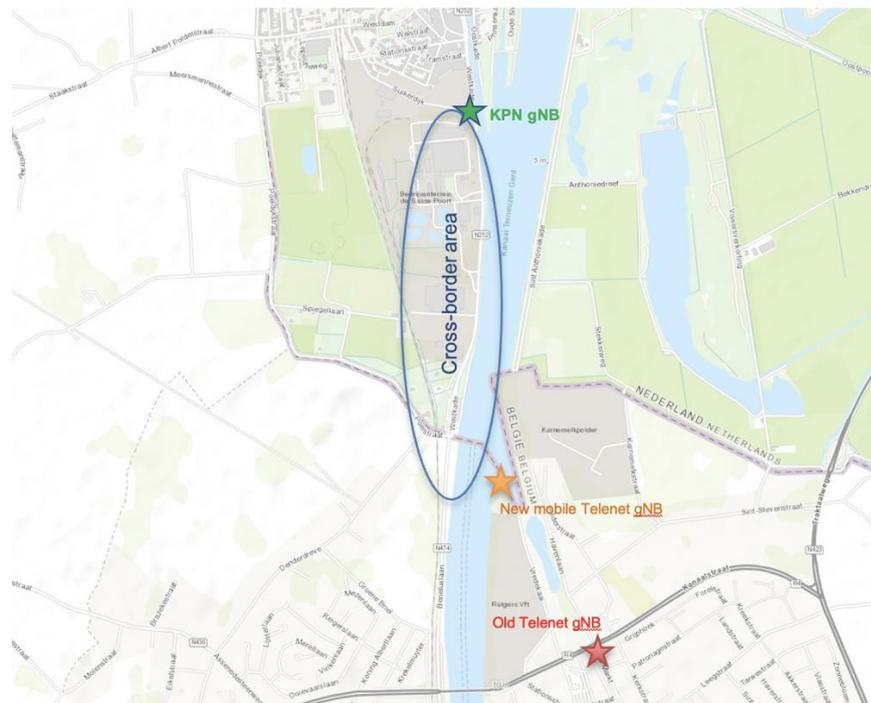
Figure 7 Cross-border area and locations of gNBs; Old Telenet gNB is located in the City Center area where EF3 has been tested (results for this location presented in Annex).
