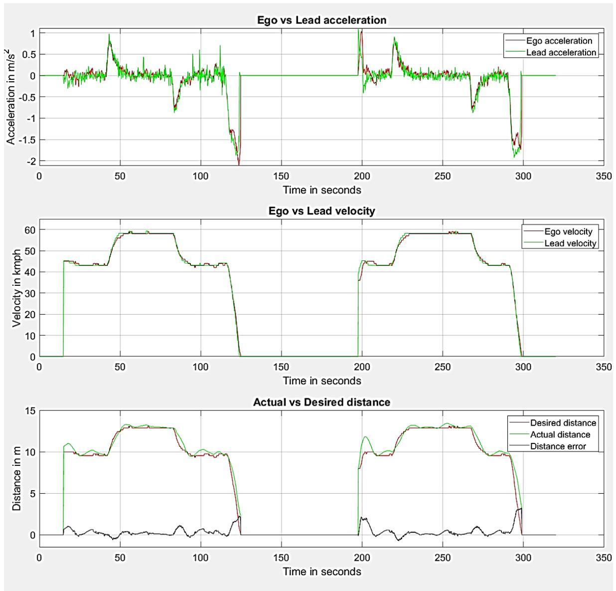
Figure 9 Test results of CCAC-based platooning in Vlissingen.
