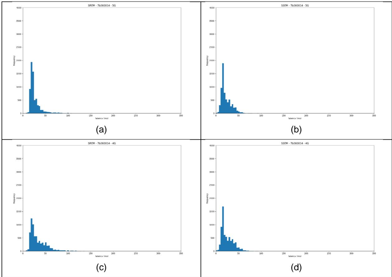
Figure 55 iTLC K0038 bar graphs latency 5G (a,b) /4G (c,d) SREM (left) SSEM (right).
