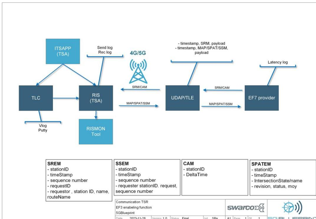
Figure 48 Test environment for EF3.
