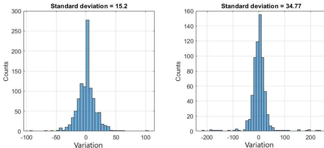
Figure 18 Histograms of the delay variation in [ms]. Left: successful test, Right: unsuccessful test.
