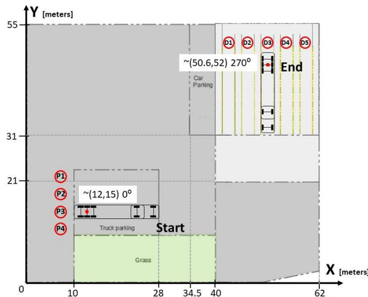
Figure 13 Top view of autodocking test at MSP Onions test site.
