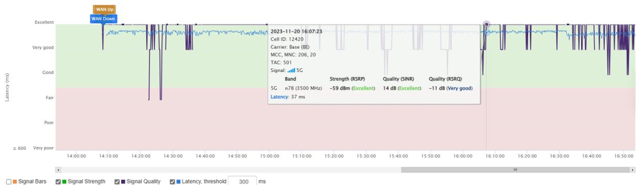
Figure 34 5G SA signal quality and latency during dry-run test in T2.8.
